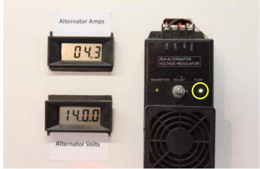
Note: Float phase, Green LED on and battery at 14.00 volts
