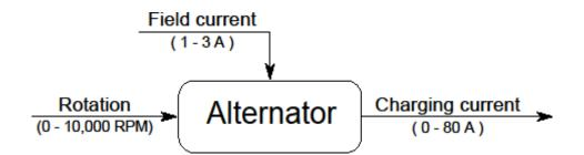
The purpose of an alternator regulator is to continuously adjust the field current in order to maintain a desired battery voltage. So it is the *field current* that is being controlled in order to set a *charging current*, which in turn establishes a desired *battery voltage*. Confusing I know.
