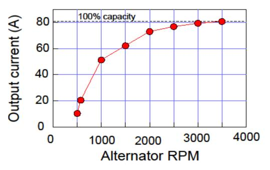
You need to calculate what your lowest cruising rpm is and arrange your pulley size to ensure your alternator is producing the best possible output.
