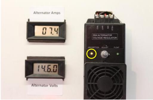
Note: Absorption phase, Yellow LED on and battery at 14.60 volts
