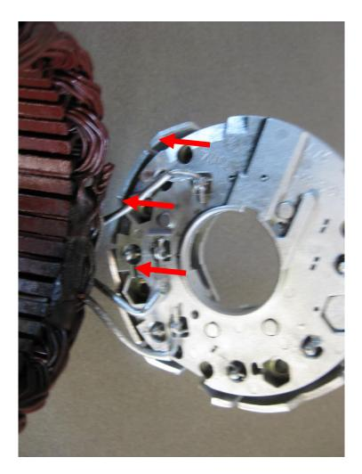
This is the rectifier plater and you need to desolder these three wires and solder onto the new one.
