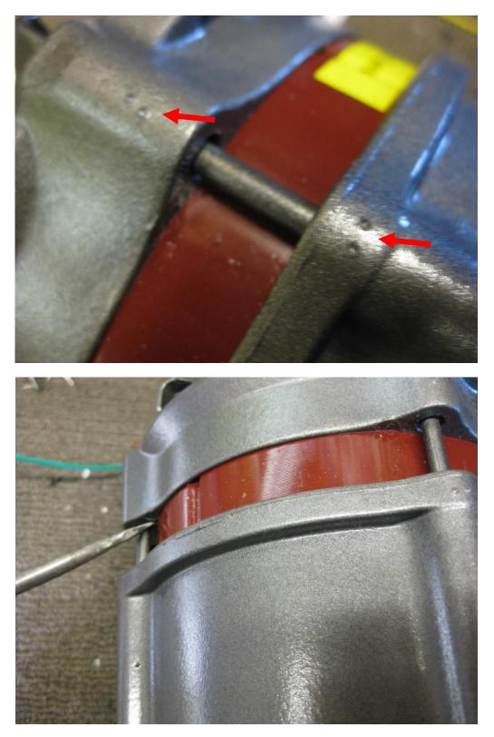
Use a screwdriver, one either side and coax the rear bearing out of the rear case, sometimes you might need to tap the forward case half to get a gap.
