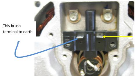
Run a wire out for Positive switching ZM6 FIELD
