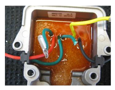
Insulate the two green wires from making electrical contact with anything inside the unit
