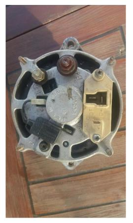
If the internal tang which connects the D+ terminal to the brush block is broken off, see if one of the two spade terminals are common with the D+, i.e. use your multimeter to check for continuity
