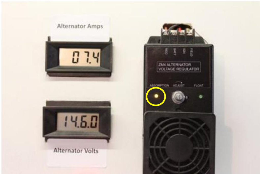
Absorption Phase: Yellow LED ON and battery at 14.60 V
