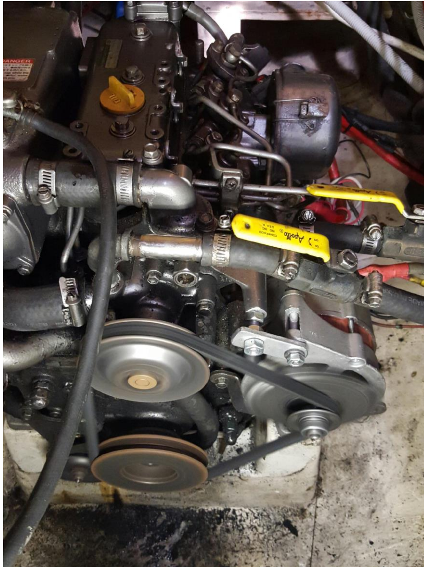
Photo 2: shows a Bosch 120-amp alternator running on a Yanmar 4jh3e engine
