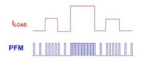
Graph showing pulse frequency modulation versus load.
