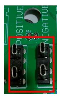
4/ On the top left side there are two fuse holders being Left side for positive switching alternators, and the right-hand fuse holder is for negative switching alternators. (Default P)
