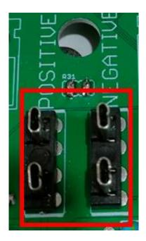
4/On the top left side there are two fuse holders being Left side for positive switching alternators and the right-hand fuse holder is for negative switching alternators.
