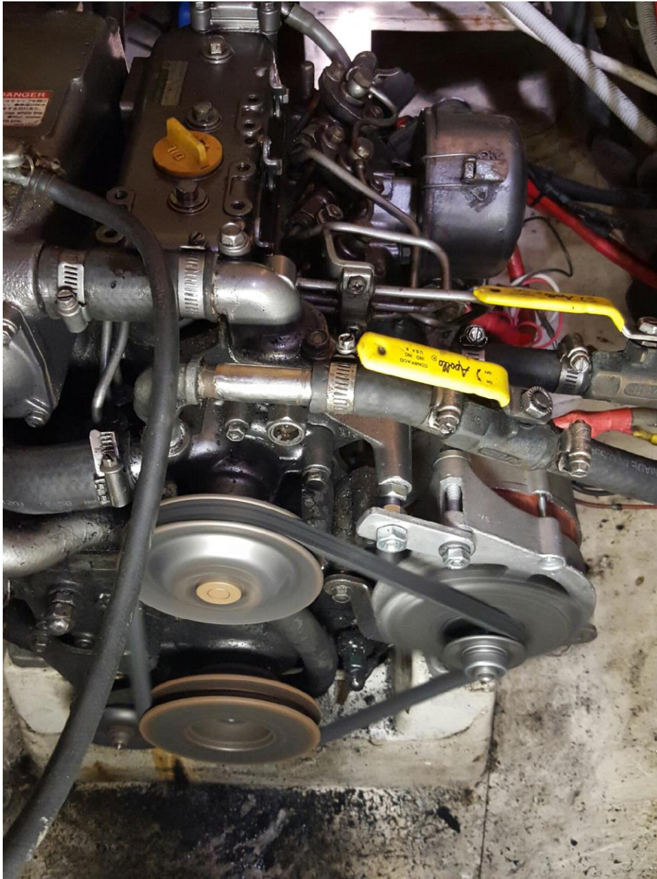
Photo 2: shows a Bosch 120 amp alternator running on a Yamnar 4jh3e engine
