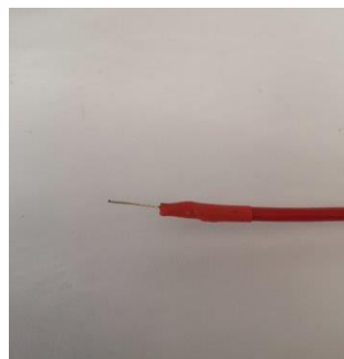
Solder a 1mm wire onto a larger wire to fit connector block correctly
