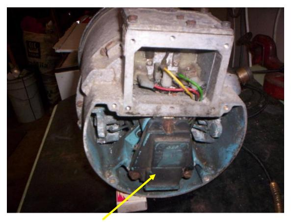
Remove this internal regulator and associated wires
